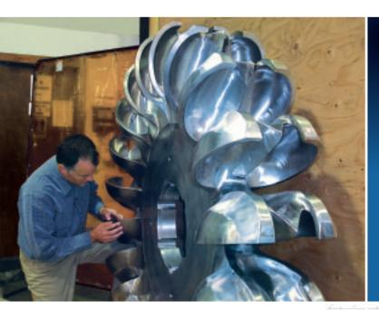
Every Canyon Hydro turbine undergoes extensive inspections and non-destructive testing. Here, Canyon Chief Engineer Brett Bauer inspects a Pelton runner destined for PG&E's 1,880 kW Phoenix project in California, with a net head of 308.75 meters (1013 feet).
