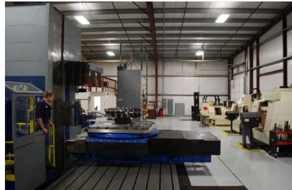
Canyon Hydro’s CNC Center features a 7-axis computerized milling machine with capacity for objects up to 36 feet long, 16 feet diameter and 25 tons.
