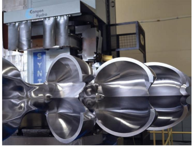
Canyon's CNC machines are equipped to address the unique requirements of hydro turbines. The special articulating arm shown above is able to reach into difficult sections to machine complex profiles.
