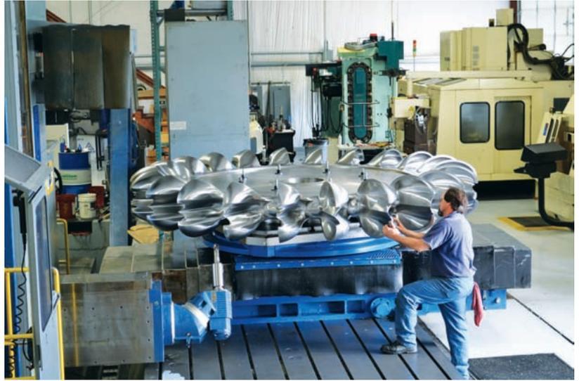
Canyon Hydro's 7-axis CNC milling machine accommodates components up to 5 meters diameter. The rotary table supports up to 15 tons. The 7MW Pelton runner shown on the machine has a diameter of 3.4 meters and weighs 21,000 pounds.
