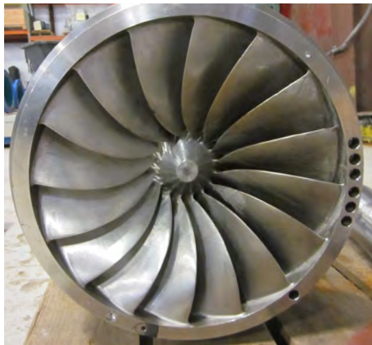
Canyon Hydro makes runners for turbines that turn water flows into electricity. Photos courtesy of the company.
