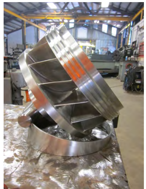
Canyon Hydro makes runners for turbines that turn water flows into electricity. Photos courtesy of the company.
