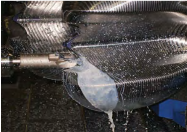
Most of the contour, roughing and finishing, is done with the large standard Ingersoll ProBall indexable ball mill.
