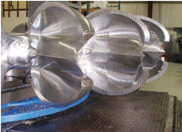
Finished buckets in the foreground (left center) have a 32- \mu m surface finish, achieved despite extremely long reaches throughout the seven-axis contour- milling operation. Standard 2" (51-mm) Ingersoll ProBall ball mill with side-cutting inserts handles both roughing and finishing.
